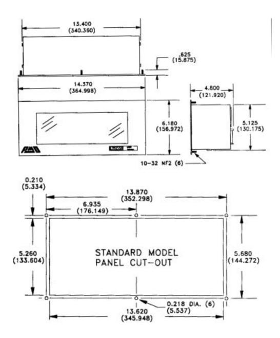
**Figure A.3** Panel Cut-Out and Outline Dimensions for the Standard Model PMD 300S.
