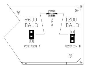
Figure 2-11. PMD 300S Jumper JP3 Location and Baud Rate Settings.
