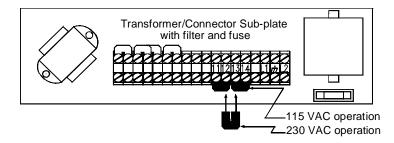
**Figure 2-16.** PMD 3000/3500 Transformer/Connector Sub-Plate Jumper Settings for 115/230 VAC Operation.
