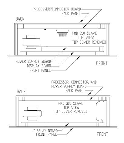
Figure 2-13. PMD 200S/PMD 300S PC Board and Transformer Locations.
