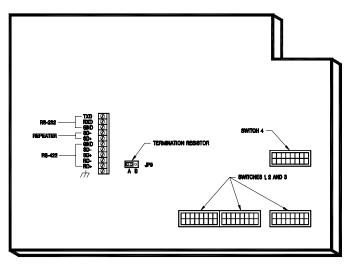
Figure 2-5. PMD 3000 and PMD 3500 Control Board Components.
