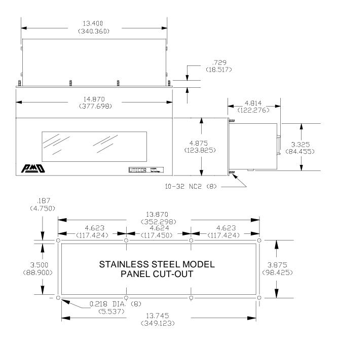
**Figure A.2** Panel Cut-Out and Outline Dimensions for Stainless-Steel Model 2-Line Display.
