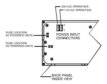
**Figure 2-15.** PMD 300S Processor/Communications Board with Power Input Connector and Fuse Locations.
