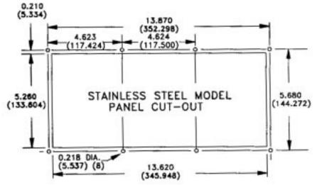
**Figure A-4.** Panel Cut-Out and Outline Dimensions for the Stainless-Steel Model PMD 300S.
