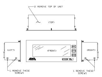
Figure 2-9. Removing the Top Cover - PMD 200S/300S.
