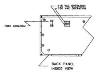
**Figure 2-14.** PMD 200S Processor/Communications Board with Power Input Connector/Fuse Locations.
