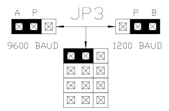
Figure 2-12. PMD 3000 Jumper JP3 Baud Rate Settings.
