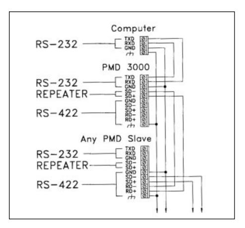
Figure 2-7. RS-232 Interfacing.
