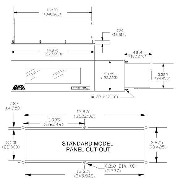
**Figure A-1.** Panel Cut-Out and Outline Dimensions for Standard Model 2-Line Display.
