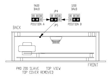
Figure 2-10. PMD 200S Jumper JP5 Locations and Baud Rate Settings.
